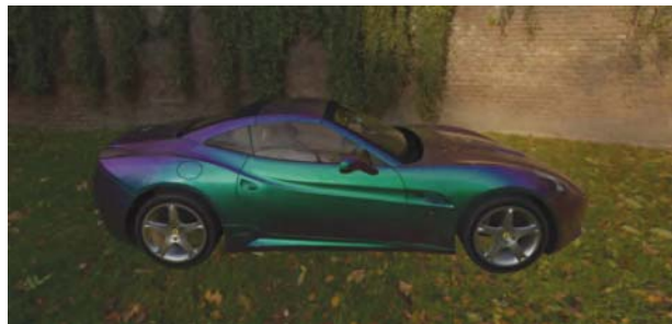
Figure 1.32 Simulation of an interference pigment coating. Source: From Musbach (2016).
